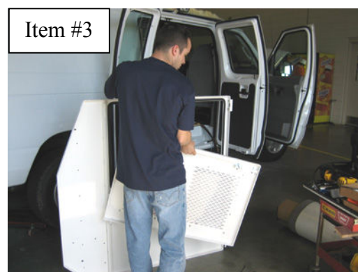
Remove Emergency Exit Hatch from Front Bulkhead to ease installation
